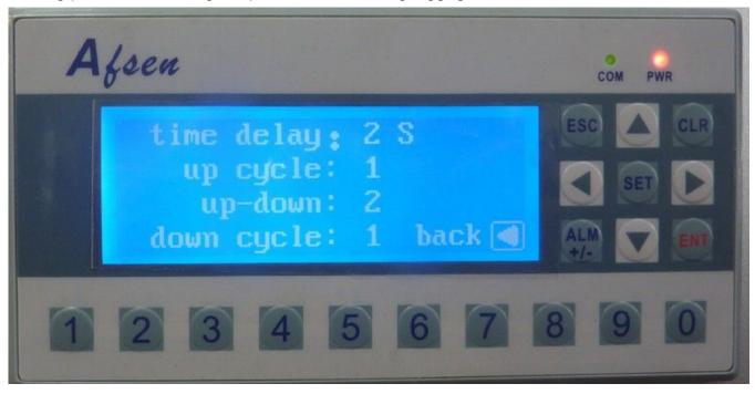
"time delay" setting the time delay when the film system arrive to the highest position
