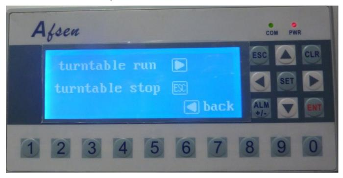
"Turntable run": press the button, the turntable will run
